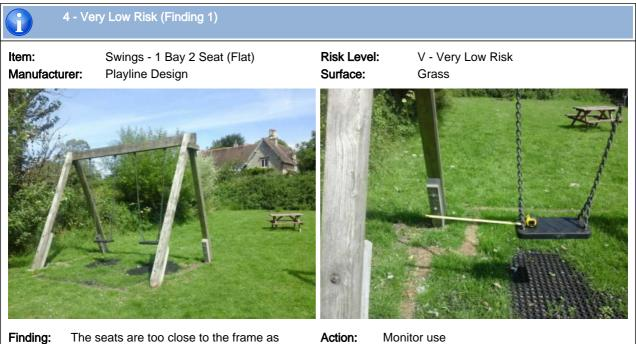
The seats are too close to the frame as defined in BS EN 1176 Part 2; this is a low risk failure and no remedial action is required
